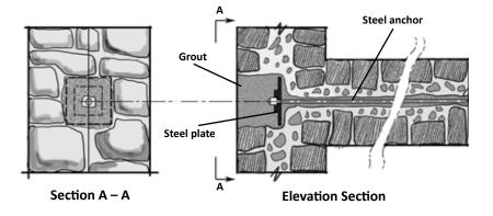
Figure 4.12 Installation of post-tensioned steel anchors to enhance connections between the intersecting walls (source: Maffei et al. 2006)
