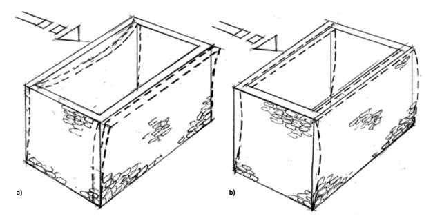
Figure 2.5 Masonry building during earthquake shaking: a) loosely connected walls without slab at the roof level, and b) a building with wellconnected walls and a roof slab (source: Tomazevic 1999)
