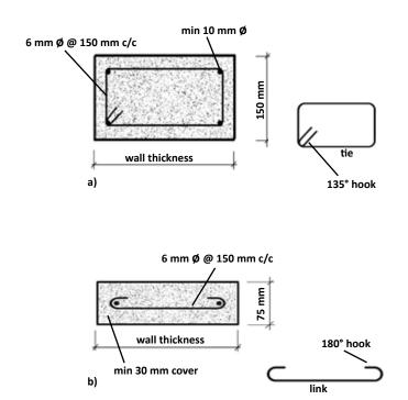
Figure 3.17 RC band cross-section: a) a band with four bars and ties, and b) a band with two bars and links
