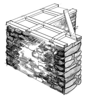
Figure 3.21 Timber band with a knee-brace at the corner
