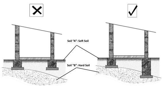
Figure 3.37 Different foundation depths are required for building sites with variable soil properties (source: GOM 1998)
