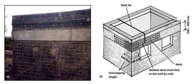
Figure 4.8 Construction of a reinforced concrete bandage: a) a retrofit application in Maharashtra, India and b) concept (source: GOM 1998)
