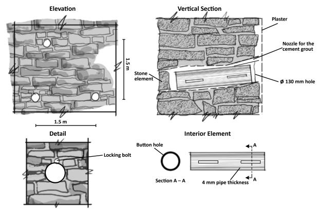
Figure 4.21 Installation of though-wall anchors in stone masonry walls after the 2002 Molise, Italy, earthquake (source: Maffei et al. 2006)
