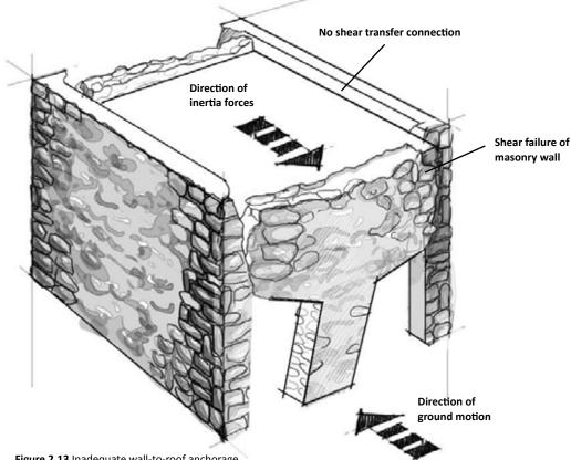
Figure 2.13 Inadequate wall-to-roof anchorage
