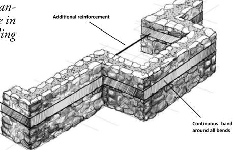
Figure 4.9 Continuing a bandage in re-entrant walls (source: R. Desai)
