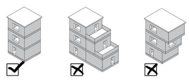
Figure 3.5 Building irregularity in vertical direction: regular buildings are recommended, and buildings with setbacks or overhangs are not.
