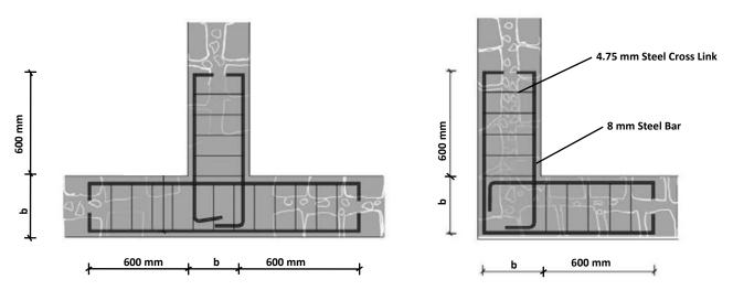
Figure 3.33 Wall stitches made from reinforced concrete with steel reinforcement (adapted from: Bothara et al. 2002)
