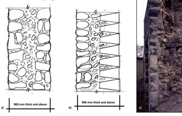
Figure 1.28 Stone masonry walls in Maharashtra, India: a) an uncoursed random rubble stone masonry wall (source: CBRI 1994); b) a semidressed stone wall with an exterior wythe built using wedge-shaped dressed stone (Source: CBRI, 1994), and c) an example of a semi-dressed stone wall (photo: S. Brzev)
