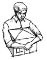
Figure 3.7 A seismic band acts like a belt (adapted from: GOM 1994)
