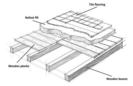
Figure 1.10 Typical floor construction in Italy with wooden beams and planks, ballast fill, and tile flooring (source: Maffei et al. 2006)
