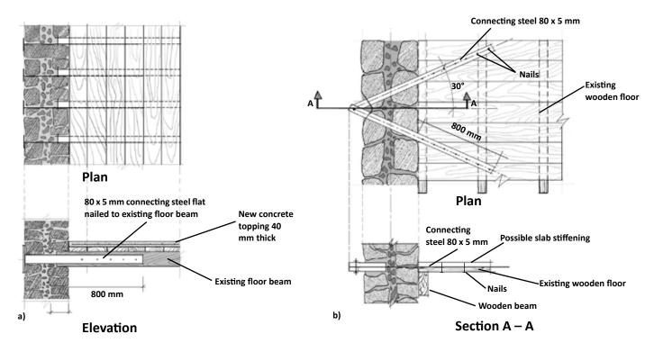
Figure 4.13 Steel straps for wall-to-floor anchorage: a) floor beams perpendicular to the wall, and b) floor beams parallel to the wall (source: UNIDO 1983)
