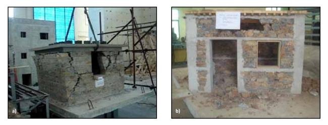
Figure 2.12 Damaged models at the end of the test: a) failure of model SM1, and b) model SM3 at the end of the experiment (source: Ali et al. 2010)
