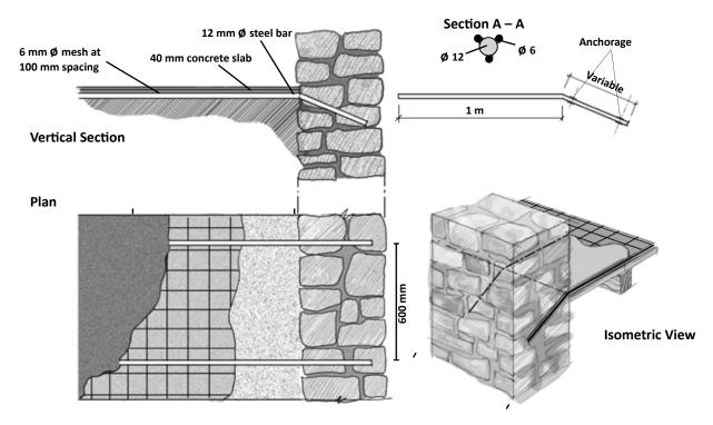
Figure 4.16 Wall-to-floor anchorage with steel dowels embedded into the wall (source: Maffei et al. 2006)
