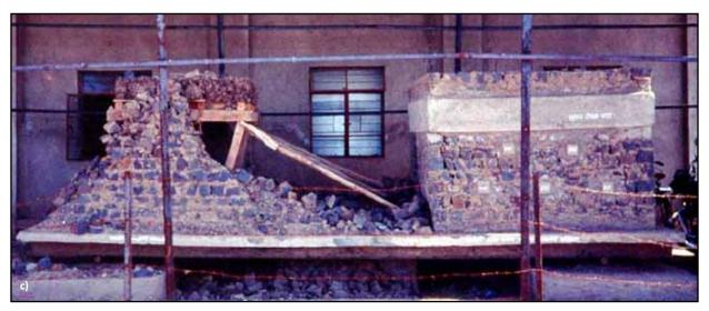
Figure 4.1 Verification of seismic retrofitting methodology for stone masonry buildings through shake-table testing: a) strengthened (retrofitted) model, b) unstrengthened model after testing, and c) models at the end of the experiment (unstrengthened model shown on the left) (source: GOM 1998)
