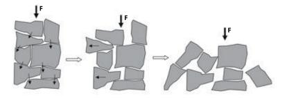
Figure 2.36 Detail of wall failure caused by irregular stones (source: Bothara and Hiçyılmaz 2008)
