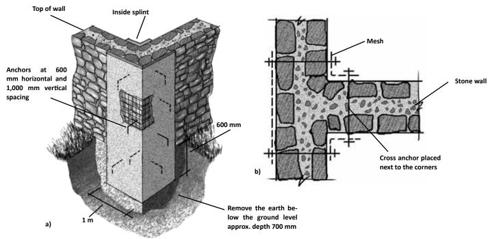
Figure 4.10 Strengthening of intersecting walls using splints : a) a concept, and b) anchorage - anchor bars tying splints on both sides of wall (source: GOM 1998)
