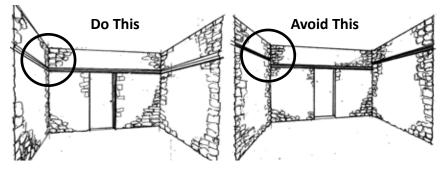
A seismic band must be continuous, like a loop or a belt.
