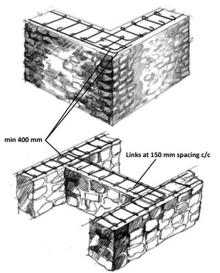
Figures 3.16 Reinforcement layout in RC bands (adapted from: GOM 1998)
