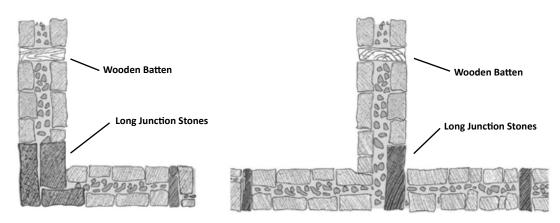
Figure 3.30 Placement of long stones at wall intersections (adapted from: Bothara et al. 2002)
