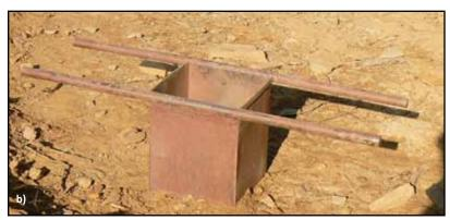
Figure 3.45 Measuring concrete materials: a) proportioning concrete ingredients using a measuring box, and b) a measuring box (photos: Smart Shelter Foundation)
