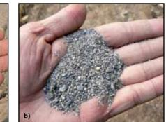
Different types of sand and their uses are illustrated in Figure 3.42. If the sand is too coarse, small pebbles must be sieved out. These pebbles could be added to aggregate for concrete construction. Sand from the sea or ocean should not be used due to the presence of salt (chlorides), which causes corrosion of steel reinforcement.
