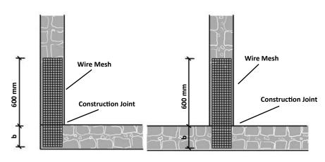
Figure 3.31 Construction of stitches made from wire mesh embedded in mortar at the wall intersection (adapted from: IAEE 2004)
